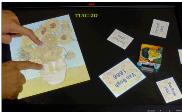
Figure 13: Chronicle demo that can support tangible and multi-touch interaction simultaneously
