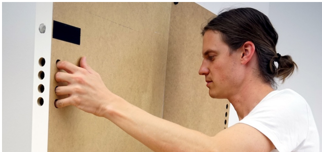
Figure 6: Finger holes enable actuators to lift boards easily
