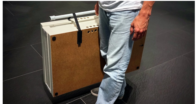
Figure 8: Boards collapse into a 90x55x20cm package that human actuators can carry like a suitcase.
