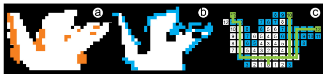
Figure 9: VRoamer pre-processes the global map by (a) taking a snapshot, (b) labeling boundaries between walkable (white) and unknown (black) areas as portal (blue) and (c) finding shortest paths (green, selected for clarity) to those portals.
