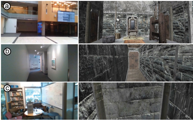
Figure 2: VRoamer (a) places pre-authored rooms when there is a space in the real world, (b) generates corridors to connect to unknown areas, and (c) shows closed virtual rooms when detecting dead-ends.
