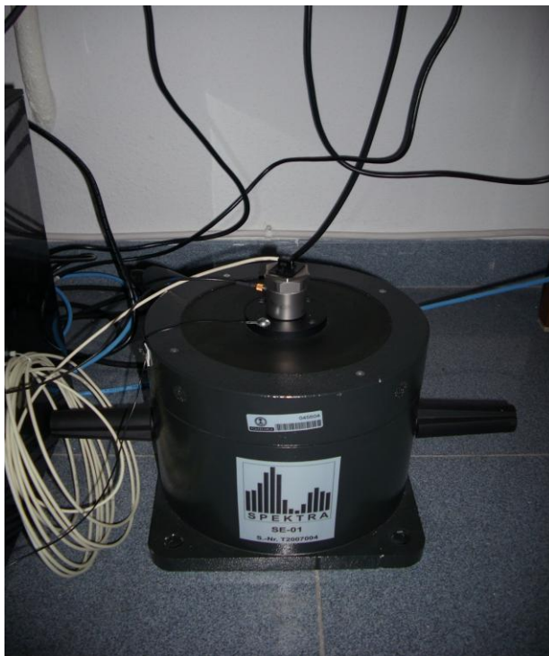
Figure 4. Experimental setup: vibration control system SRS-35, power amplifier PA-14-180, vibration exciter SE-1, and Standard-PC.
