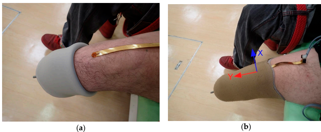
Figure 13. Photographs showing how the sensor was attached to the stump in the prosthesis liner: (a) Sensor head of the shear force sensor was attached to the tibial tuberosity with a double-sided adhesive tape, and the measurement started; and (b) The prosthesis liner was fully donned.
