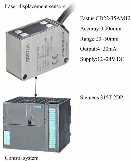
Figure 10. The hard structure of data collect system for laser displacement sensors.
