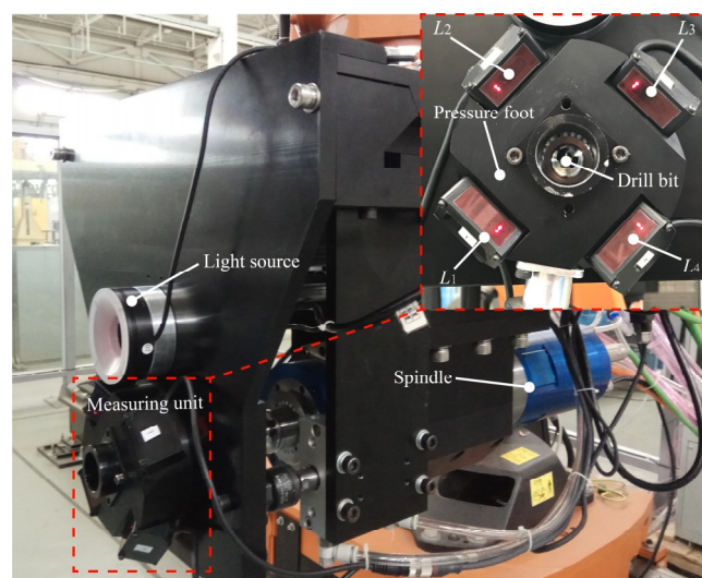
Figure 3. The installation of four laser displacement sensors.
