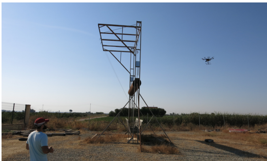
Figure 4. The outdoor setting for real flights using the UAV in Figure 3, the obstacle to avoid, and the safety pilot.
