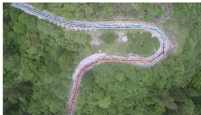
Figure 9. Road line fitting results. The thick solid line represents the centerline of the road, and different colors are used to distinguish different road units. The large colored circles represent the control points of each road unit.
