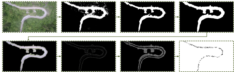
Figure 2. Method of extracting star points from an image of a road: brightness thresholding, morphological opening operation filtering, obtaining the ROI contour, extracting the ROI area, Laplacian texture sharpening, sharpening image binarization, and obtaining the star points.
