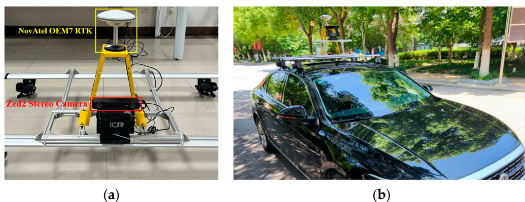
Figure 8. Image (a) shows the onboard experimental platform, with the ZED2 stereo camera in the red box and the RTK device in the yellow box, and (b) shows the actual installation effect of the vehicle-mounted experimental platform.
