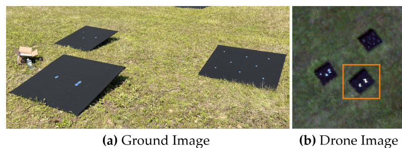
Figure 4. (a) Primary site for G-SCALE where point targets were deployed for radiometric and spatial testing. (b) HSI image (RGB bands shown) over the point targets where the orange box highlights the targets used in the analysis.
