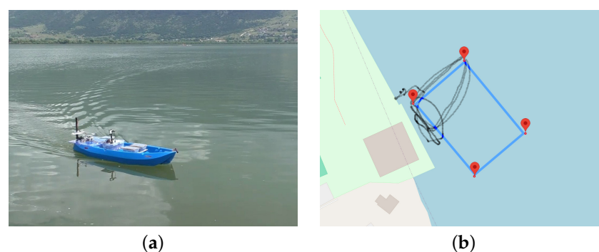
Figure 15. (a) Trial at the lake Pamvotis, Ioannina. (b) GPS log from the autopilot system test at the lake Pamvotis, Ioannina. On the day of the test there were some pondweed present. Hence, other two waypoints were unreachable. This presented us with the opportunity to test the waypoint skip function.
