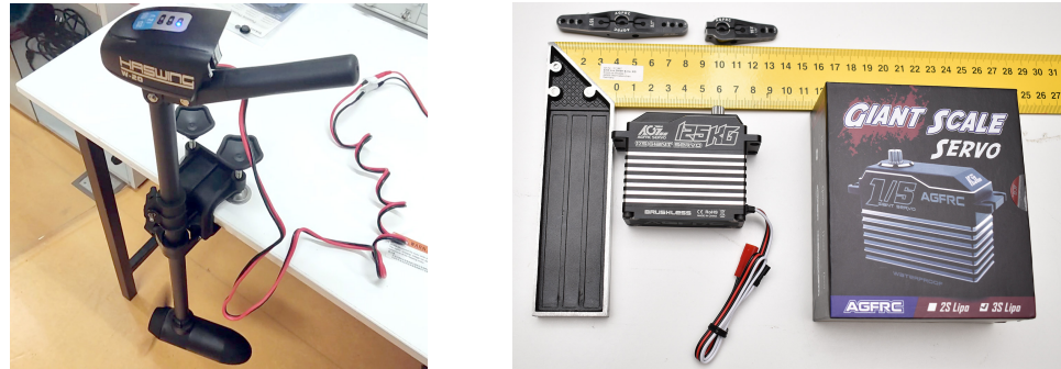
(a) Haswing W20 electric trolling motor; (b) AGFRC A280BVSW high-speed servo
