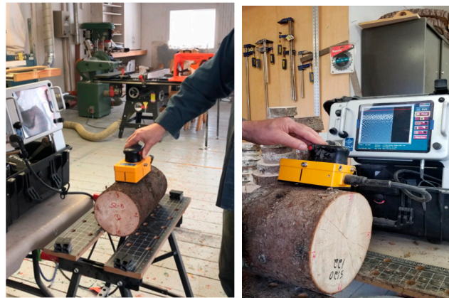
Figure 2. GPR signal acquisition through bark.
