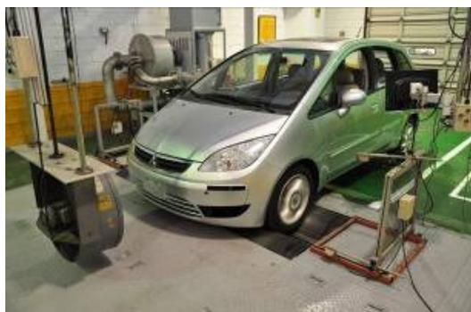
Figure 10: Emission &amp; Fuel Economy Testing Lab to LDV.
