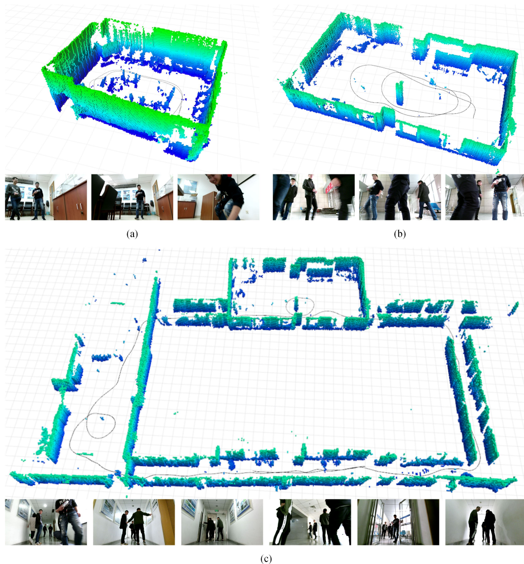
Figure 13. Results of the extension tests. (a) 8\text{ m} \times 6\text{ m} office (Voxel size: 0.05\text{ m} ), (b) 15\text{ m} \times 9\text{ m} hall (Voxel size: 0.05\text{ m} ), and (c) 37\text{ m} \times 27\text{ m} corridor (Voxel size: 0.1\text{ m} ). The black lines are the robot trajectories of keyframes.
