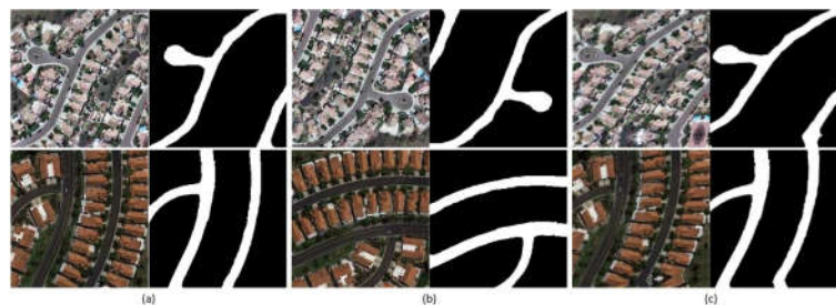
Figure 5. Morphological change methods of data augmentation: (a) Original image and its ground truth. (b) Image and its ground truth after the random flip process. (c) Image and its ground truth after the elastic deformations process.
