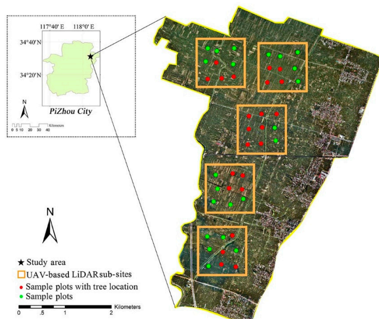
Figure 2. The black pentagram in the picture is the geographical location of the study area, the orange box is the coverage area of the unmanned aerial vehicle based light detection and ranging (UAV-LiDAR) plots, and the red dots and the green dots are fieldwork plots.
