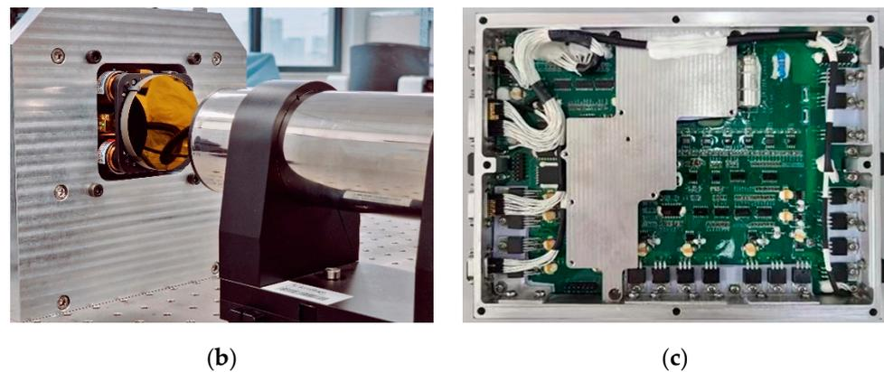
**Figure 17.** Photo of experimental platform: (a) 3D Physical Model of dual-FSM GI LiDAR tracking imaging system; (b) physical image of FSM for laser tracking system; (c) physical image of two-dimensional turntable composite axis controller.
