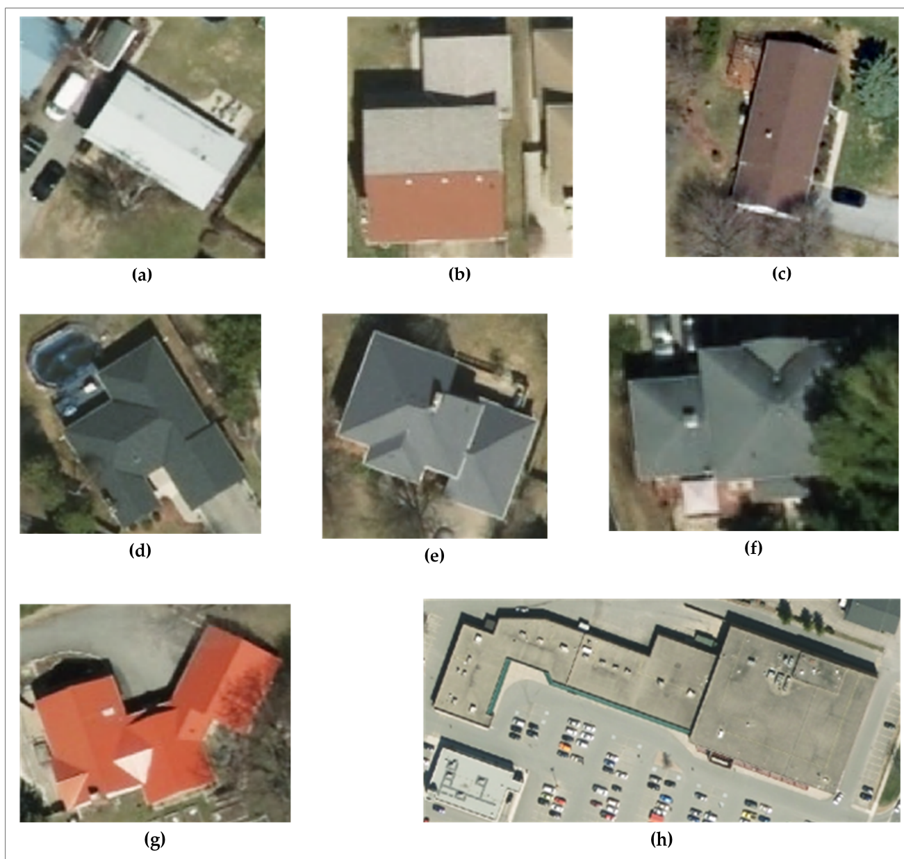
Figure 5. Sample types, shapes, and colors of the buildings available in the study area: gable roof (a–c), hip roof (d–f), complex roof (g), and flat roof (h).
