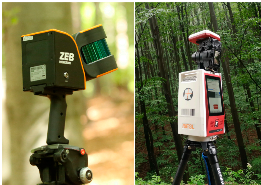
Figure 1. GeoSLAM Zeb Horizon (left) and RIEGL VZ-600i (right) during fieldwork.
