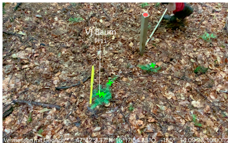
Figure 2. Screenshot from the GeoAce App (ITS Geo Solutions GmbH, Jena, Germany) during fieldwork. The green crosses mark the positions of marked trees, while the red dot marks the plot center. The positions of the surveyed trees were visualized in CloudCompare to avoid the clipping of trees smaller or larger than the predefined threshold.
