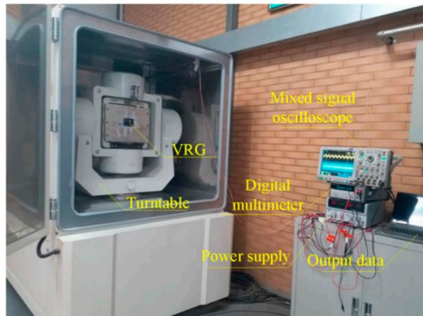
Figure 15. DUVRG scale factor test platform.
