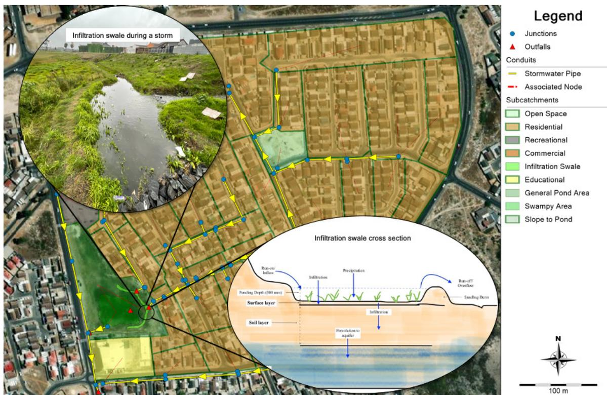
Figure 9. Post-retrofit model structure (arrows denote direction of stormwater flow).
