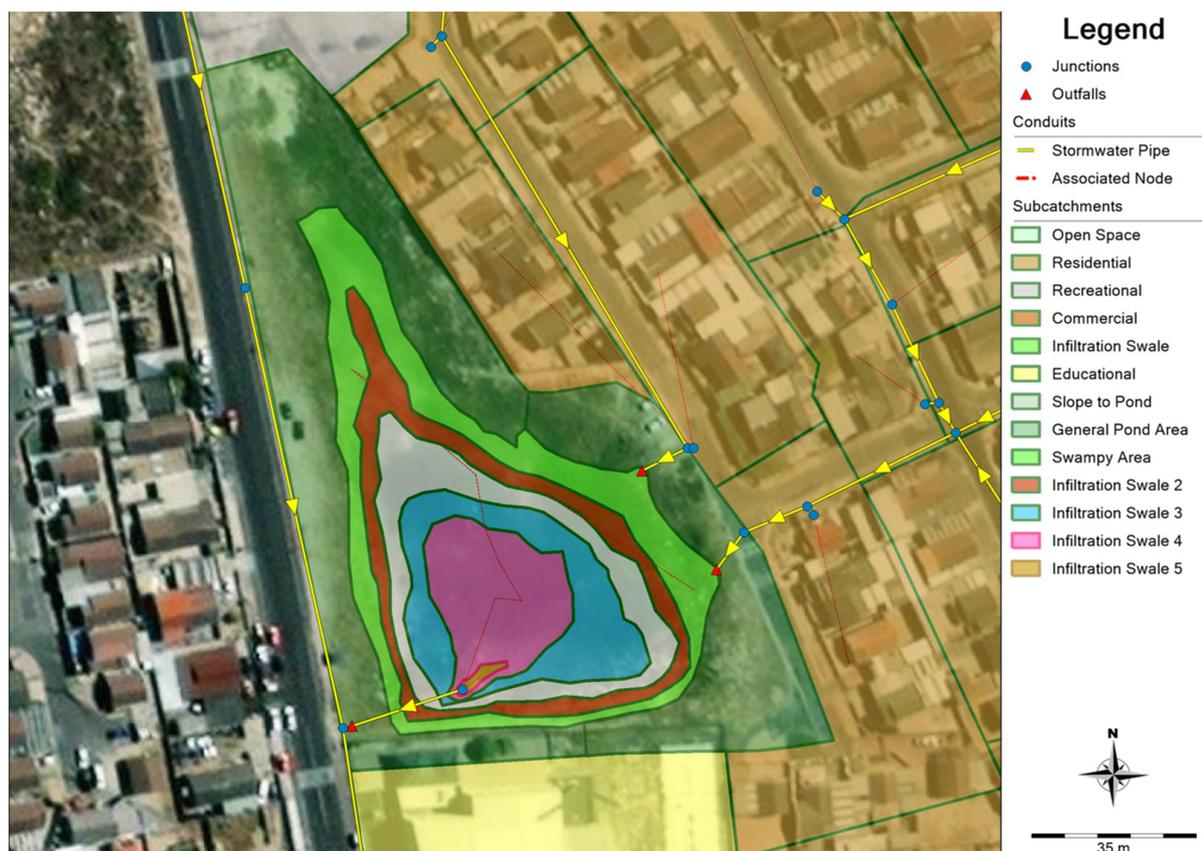
**Figure 10.** Extended LID area model structure (arrows denote direction of stormwater flow).
