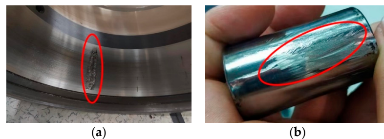
Figure 10. Physical diagram of axle box bearing fault. (a) Outer ring fault of TRB; (b) rolling element fault of CRB.
