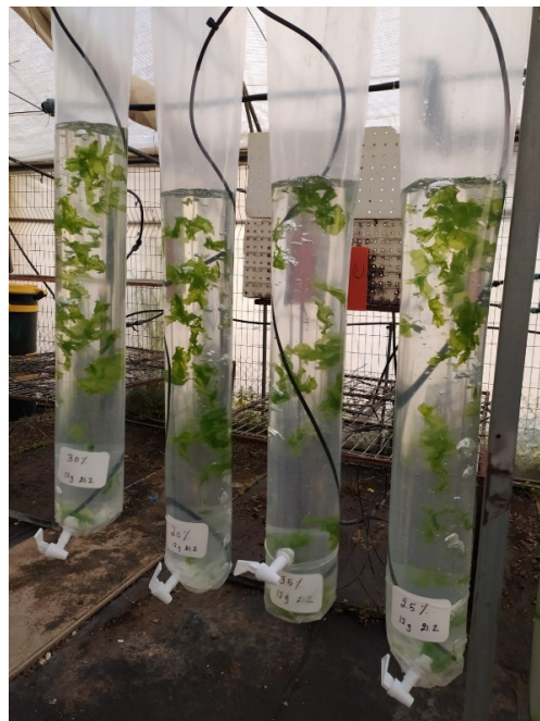
Figure 1. Ulva lactuca seaweed, cultivated in a 10 L plastic sleeve, which served as a photobioreactor, was situated in an outdoor plastic house at the Triangle Research and Development (TDRC). The cultivation conditions included an irradiance of \mu\text{mol m}^{-2} \text{ s}^{-1} , a 12/12 h light/dark photoperiod, and an artificial seawater (ASW) pH maintained at 8.2. The temperature was controlled at 25 °C during the day and 15 °C at night. A total of 12 fresh samples (3 replicates) were collected for each of the 4 treatments with ASW salinity concentrations of 2.0%, 2.5%, 3.0%, and 3.5%.
