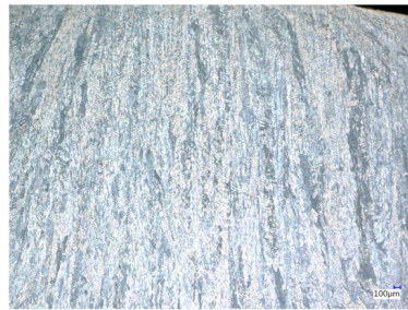
Figure 14. Microstructure of CL clad of the wheel 03.
