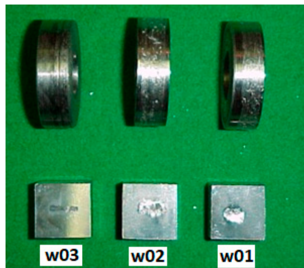
Figure 18. Tribological pairs after the 120 \text{ s}^{-1} friction test.
