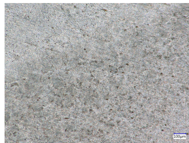
Figure 10. Microstructure of the IL to HAZ transition of round 01.
