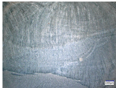
Figure 15. Microstructure of the CL to IL transition of the wheel 03.
