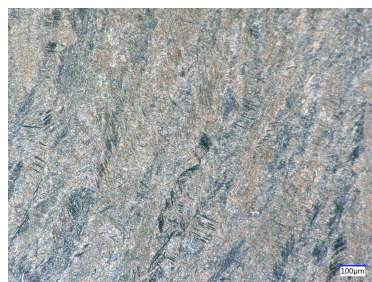
Figure 11. Microstructure of the CL clad of the wheel 02.
