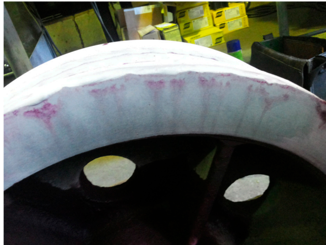
Figure 6. Running wheel w03 during capillary check—outside of rim.
