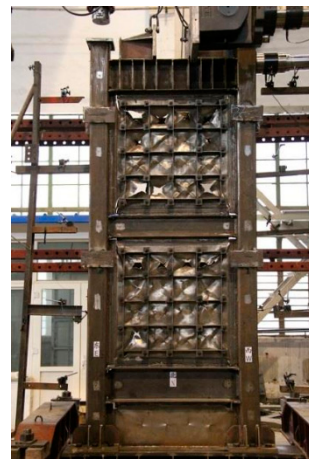
(a) Specimen overall failure
