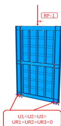
Figure 4. Boundary conditions and loads.
