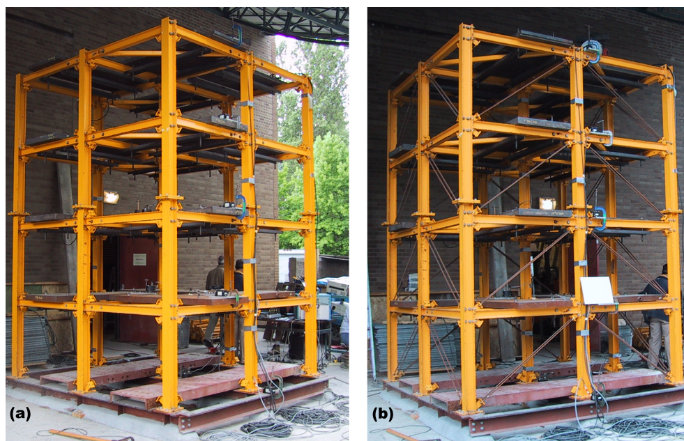
Figure 9. Yellow Frame: (a) with bracings and (b) without bracings. Source: [40].
