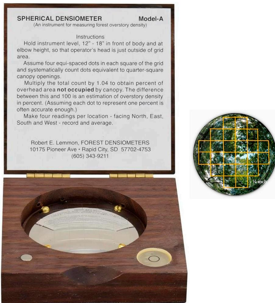
Figure 19. Spherical densiometer with over-head canopy reflection [99,100].
