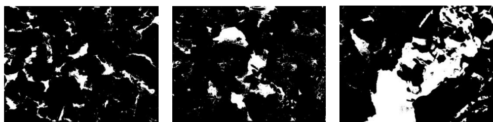
(a) S1 after 0 freeze-thaw cycles (b) S1 after 5 freeze-thaw cycles (c) S1 after 10 freeze-thaw cycles
