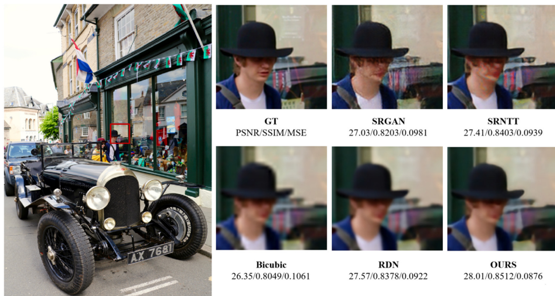
Figure 6. Visual results for the comparison on a BSD100 random image between bicubic interpolation, GT, SRGAN, SRNTT, RDN, and our model with scaling factor \times 4 .
