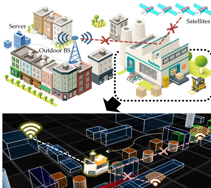
Figure 1. Illustration of the single BS-assisted JAEDE, compared with other outdoor ( upper ) and indoor ( lower ) localization techniques.
