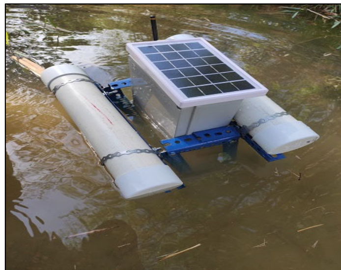
Figure 2. Prototype of a water quality monitoring station.
