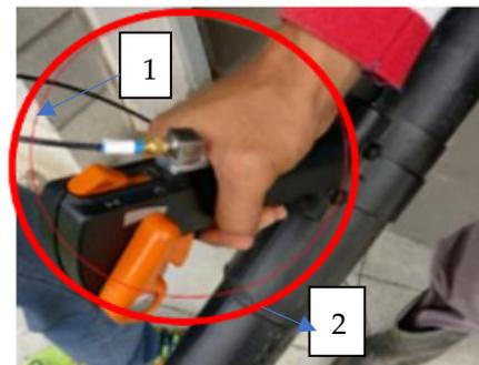
**Figure 10.** Palm adapter positioned between the hand and the tool handle (in the circle) [39].
