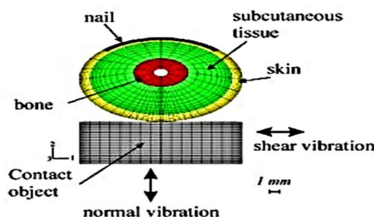
Figure 5. A two-dimensional (2D) finite-element model of a fingertip in contact with a flat surface [33].
