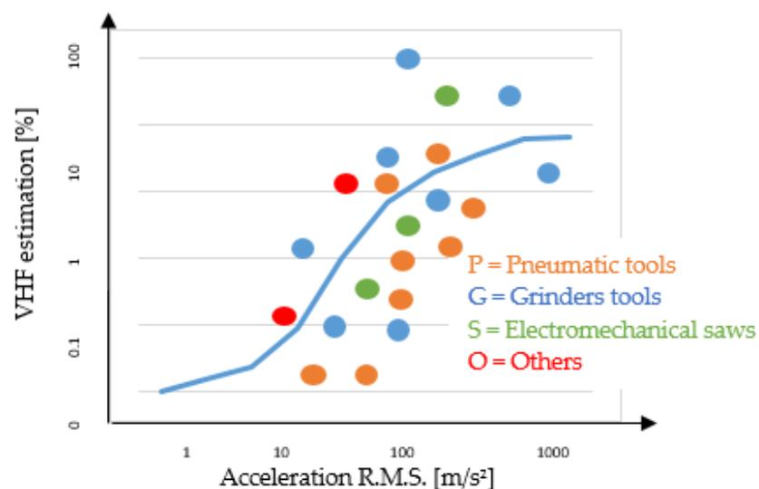
**Figure 12.** Relationship between vibration frequency, acceleration  $a_{R.M.S.}$ , and probability of white finger syndrome [1].
