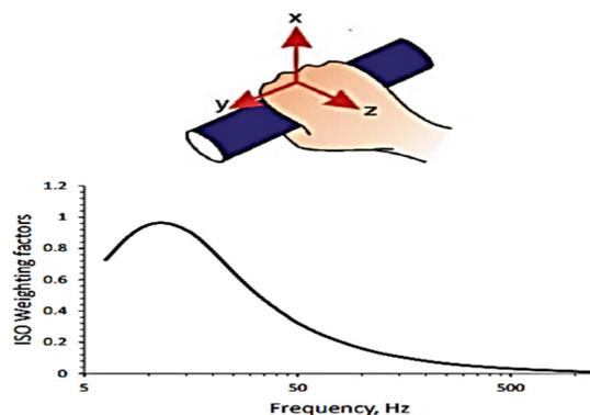
Figure 4. Diagram of the three orthogonal directions—x, y, and z—and the frequency weighting curve ( $W_h$ ) as outlined in SR EN ISO 5349-1/2003 [33].
