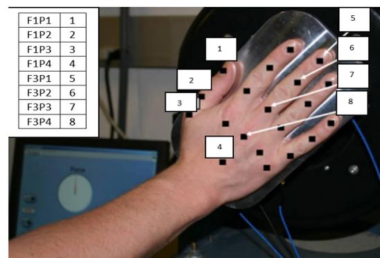
**Figure 2.** Laser scanning points on five fingers and the back of the hand [30].
