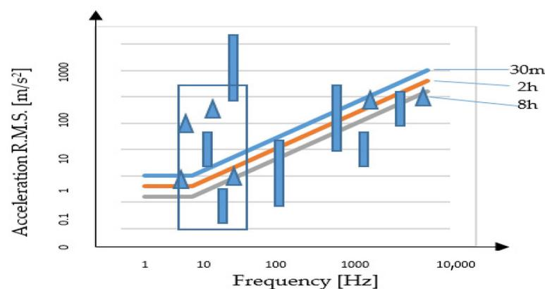
**Figure 11.** The  $a_{R.M.S}$  acceleration values at which symptoms of VWF occur [1].
