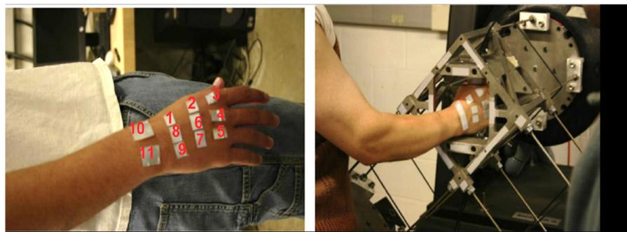
**Figure 9.** Measurement locations on the hand dorsum and pictorial view of hand–arm posture during the measurement. The arms are bent at an angle of around 90° to the original direction of the forearm [38].
