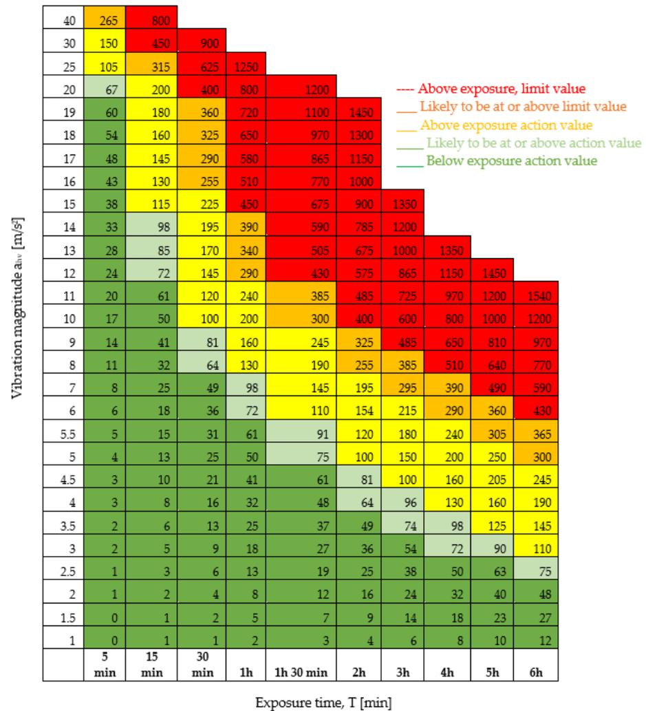
Figure 14. List of results obtained from Brandon Hire Station SHEQ [64] regarding the admitted exposure to vibration of the hand–arm system.
