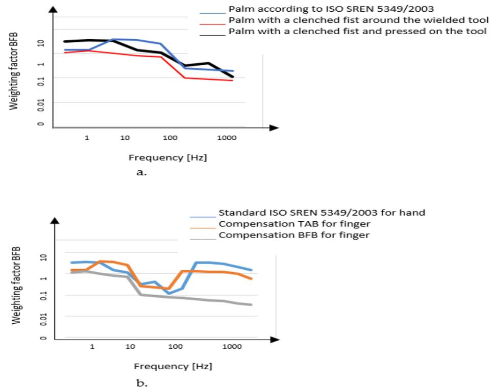
**Figure 1.** (a) BFB factors obtained for weighted frequencies [1] and (b) TAB factors obtained for weighted frequencies [1].
