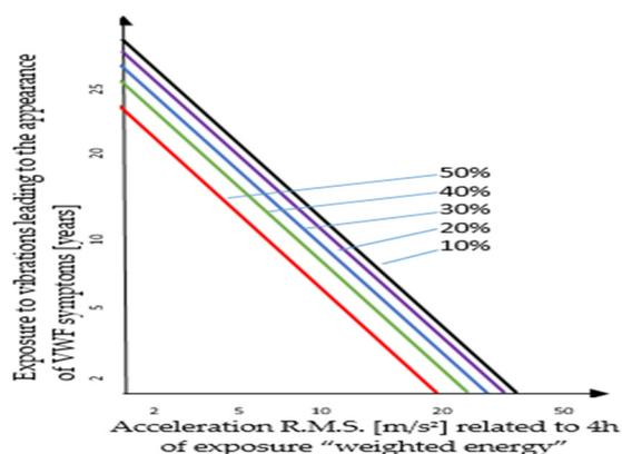
**Figure 13.** Transmission of vibrations to the hand at a daily exposure of 4 h "weighted energy" (years) and appearance probability of VWF syndrome [1].
