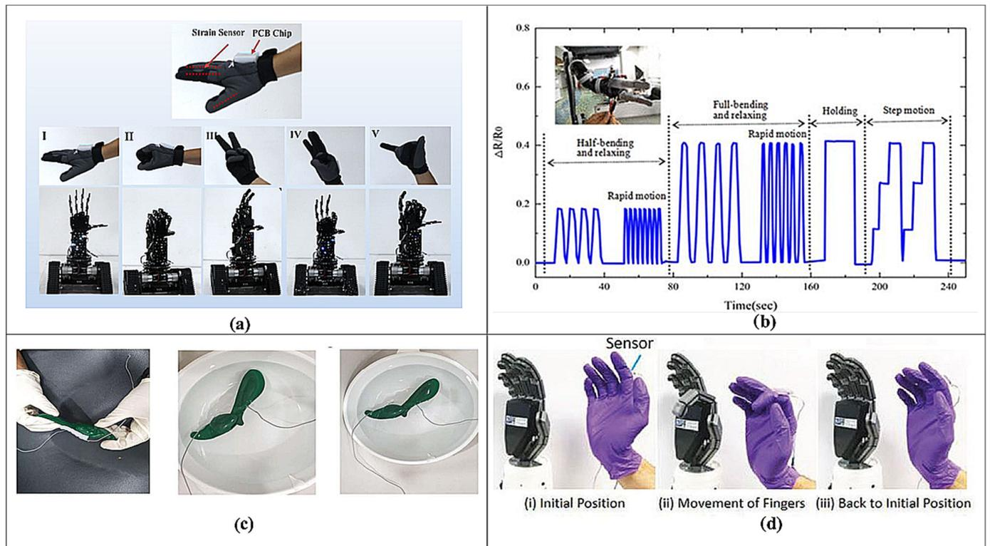
**Figure 10.** Flexible strain sensor application in robotics: (a) controlling a robotic hand from the remote position [72]; (I) original state (II) hard fist (III) bending 3 fingers (IV) bending 2 fingers and (V) bending 4 fingers (b) the sensor is attached to the robot joint to analyze the movement [77]; (c) the sensor attached to the legs under water [45]; (d) to move the robotic finger as feedback, the sensor is attached in the human finger [37].
