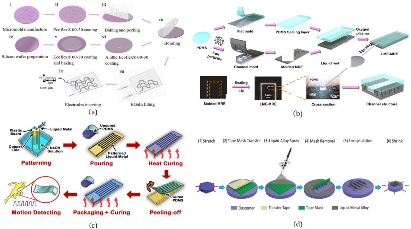
**Figure 8.** Fabrication methods to design a fluidic strain sensors: (a) a sensor designed using the soft lithographic technique [77]; (b) a sensor designed through the mold-casting method [105]; (c) a sensor fabricated using the wetting and pouring method [72]; and (d) the shrink-stretch pattern (SSP) method was used along with tape transfer and the spraying technique to design the sensor [103].
