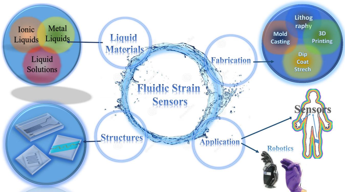
**Figure 1.** Classification of fluidic type strain sensors fabricated by exploiting either of channel structures, liquid materials, manufacturing approach, and targeted applications.
