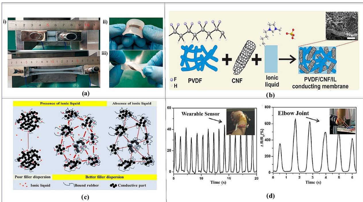
**Figure 3.** Conductive ionic based strain sensors: (a) representation of the designed strain under (i) stretching, (ii) bending, and (iii) twisting [31]; (b) the conductive material made when IL was added to the PVDF and CNF membrane [93]; (c) the schematic diagram representing the effect of IL on the bound rubber [96]; (d) the resistive change by the movement of the strain sensor [48].
