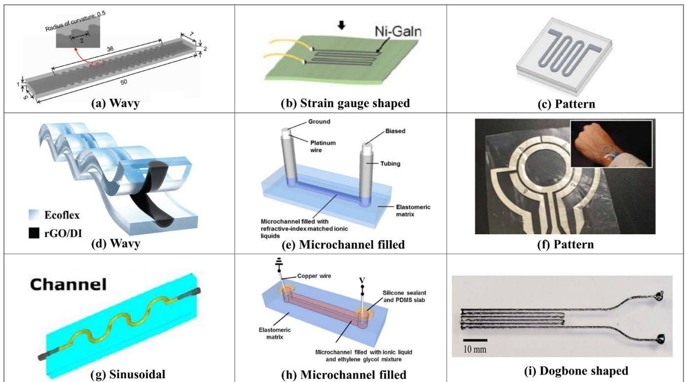
**Figure 7.** Different structures adopted by sensors to design a conductive fluidic strain sensor: (a) wavy [39]; (b) strain gauge shaped [99]; (c) pattern [100]; (d) wavy [41]; (e) microchannel filled [94]; (f) pattern structure [101]; (g) sinusoidal structure [45]. (h) Microchannel [97] and (i) dog bone shaped [104].
