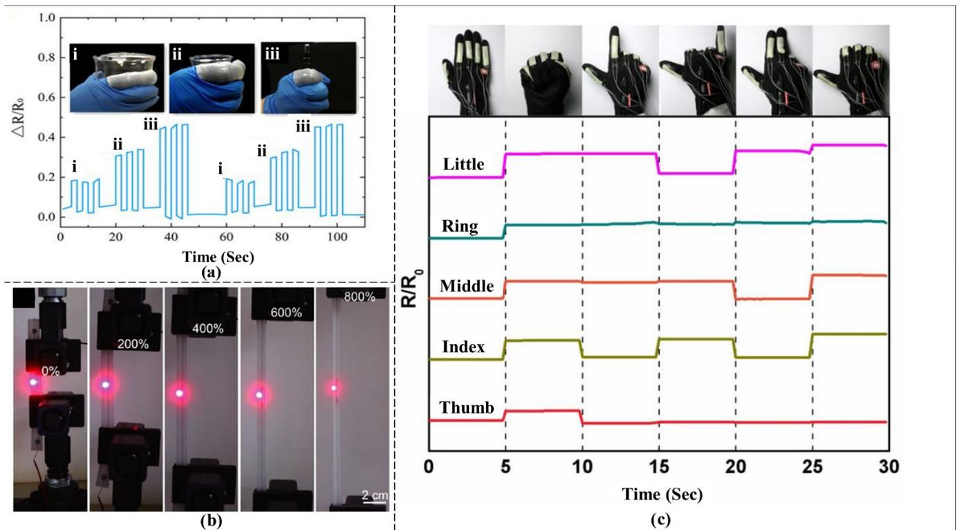
**Figure 4.** Conductive metal liquid-based strain sensors: (a) analyzing the resistance change of the sensor at different sizes [77]; (i) analyzing resistance change through bending an index finger by grabbing a large object; (ii) medium object; (iii) and small object (b) testing the stretchability at different strains [98]; (c) real-time analysis of the change in resistance by movements of the fingers [99].
