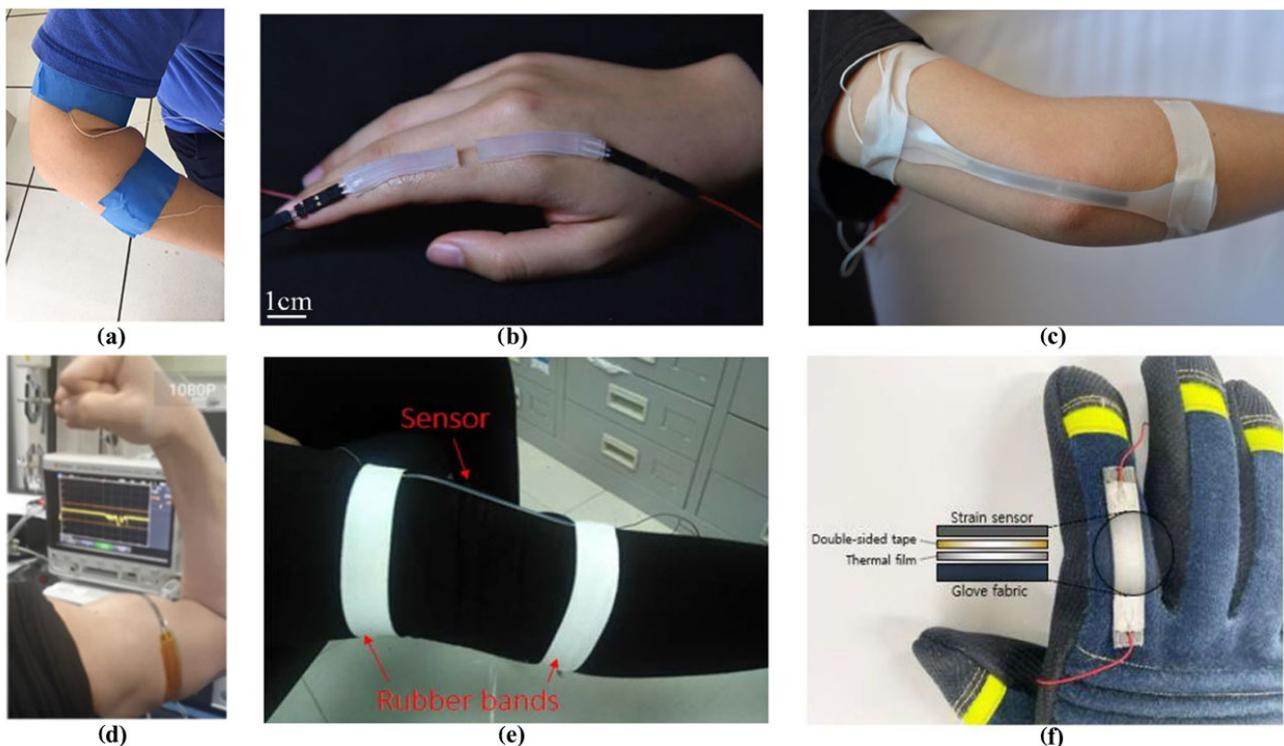
**Figure 9.** Applications of wearable strain sensors: (a) strain sensor designed to monitor movements [73]; (b) wearable strain sensor to detect finger movement [40]; (c) wearable sensor to detect elbow flexion [103]; (d) sensor worn to detect bicep muscle tuning [109]; (e) wearable sensor to detect the motion of the knee [91]; (f) attaching a sensor to a firefighter's glove to detect motion [110].
