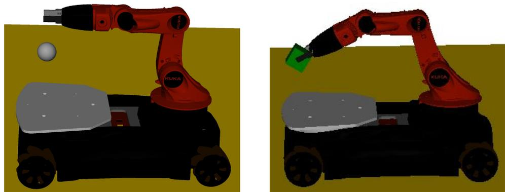
**Figure 12.** (Left) Scenario 1: A YouBot robot after releasing a free falling sphere (six DoF). The sphere will bounce on the grey plate. (Right) Scenario 3: A YouBot transporting a box with segmented simulation.
