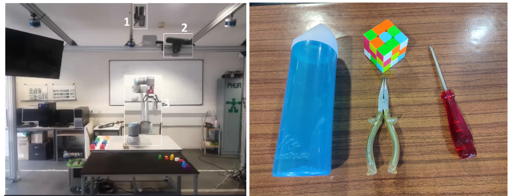
Figure 13. Experimental setup depicting the collaborative cell where the study was conducted. On the left, it features two RGB-D cameras (marked as white rectangles 1 and 2) and the UR10e COBOT (marked as white rectangle 3). On the right are the objects used to discriminate based on their grasping patterns.
