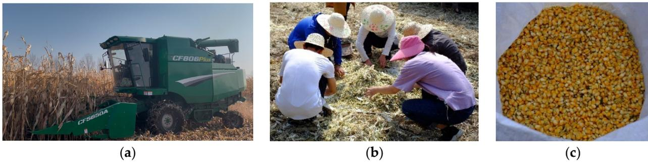
**Figure 9.** Field operation of harvester and manual collection; (a) field test of harvester material collection; (b) manual screening of lost grains; (c) grain bin contamination.
