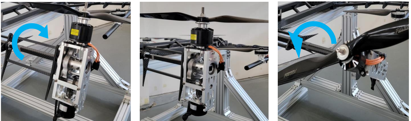
Figure 3. Tilting rotor drive mechanism and drive process.
