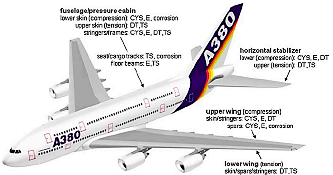
Figure 2. Engineering property requirements for the main structural areas of a transport aircraft, i.e., corrosion, fatigue, fatigue crack growth, fracture toughness. CYS = compressive yield strength; E = elastic modulus; TS = tensile strength; DT = damage tolerance properties [66]. Reproduced with permission from Springer.
