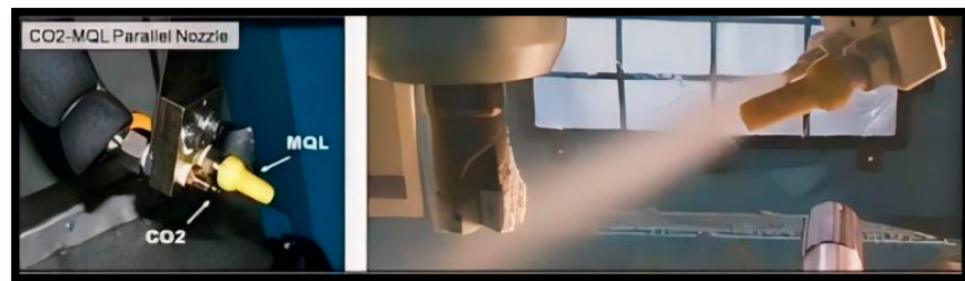
Figure 2. Cryo-MQL experimental configuration [6].
