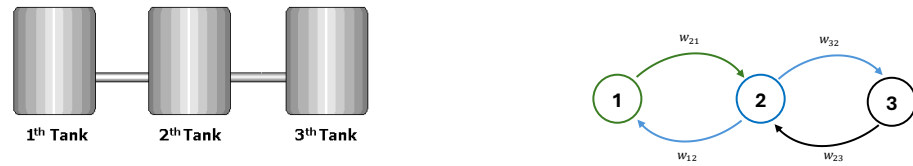
Figure 2. System of three interacting tanks without inputs/outputs (left) and its associated graph (right).
