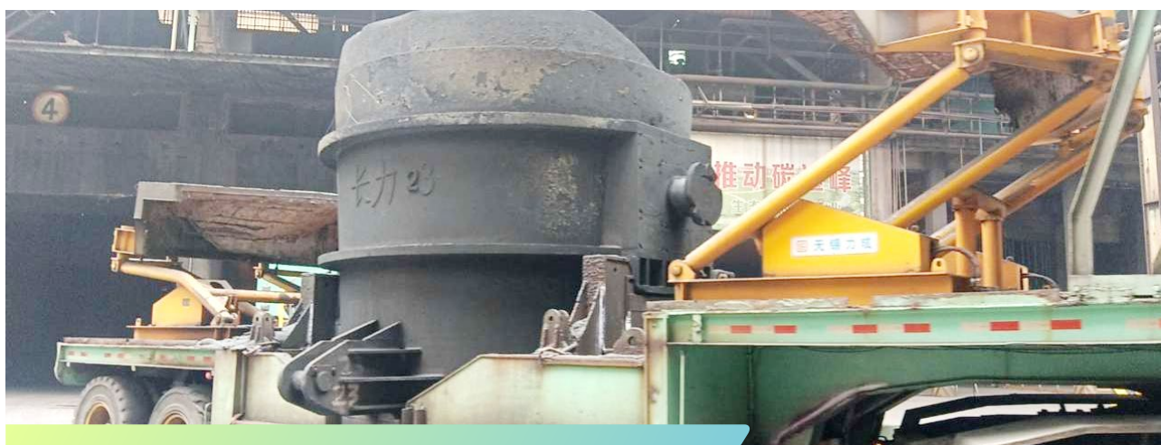
铁水车铁包加盖
