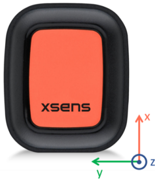
FIGURE 2. Sensor coordinate frame of the Xsens Dot
