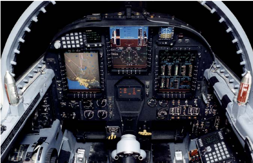
In 2000, the U-2 fleet was equipped with modern cockpit instruments, right, to replace antiquated control panels that had been in use since 1967. (Lockheed Martin)
