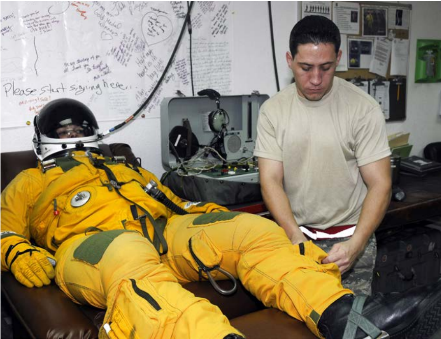
The pre-breathing ritual was the same regardless of whether the partial-pressure or full-pressure garment was worn. In upper photo, a life-support technician checks oxygen levels for Lockheed test pilot Robert Schumacher in 1957. In lower photo, TSgt. Shawn Hansen performs a similar task for Lt. Col. Brian Dickinson in 2008. (U.S. Air Force)
