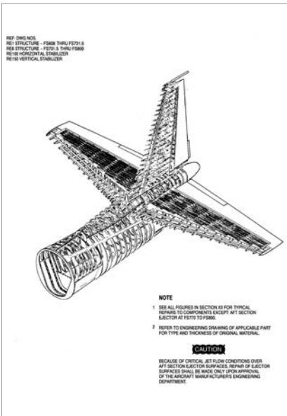
As with the fuselage and wings, the U-2 empennage was constructed from lightweight aluminum alloys. (U.S. Air Force)
