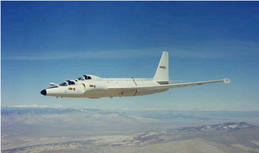
The U-2CT had an instructor's station above and behind the student's cockpit. (U.S. Air Force)
