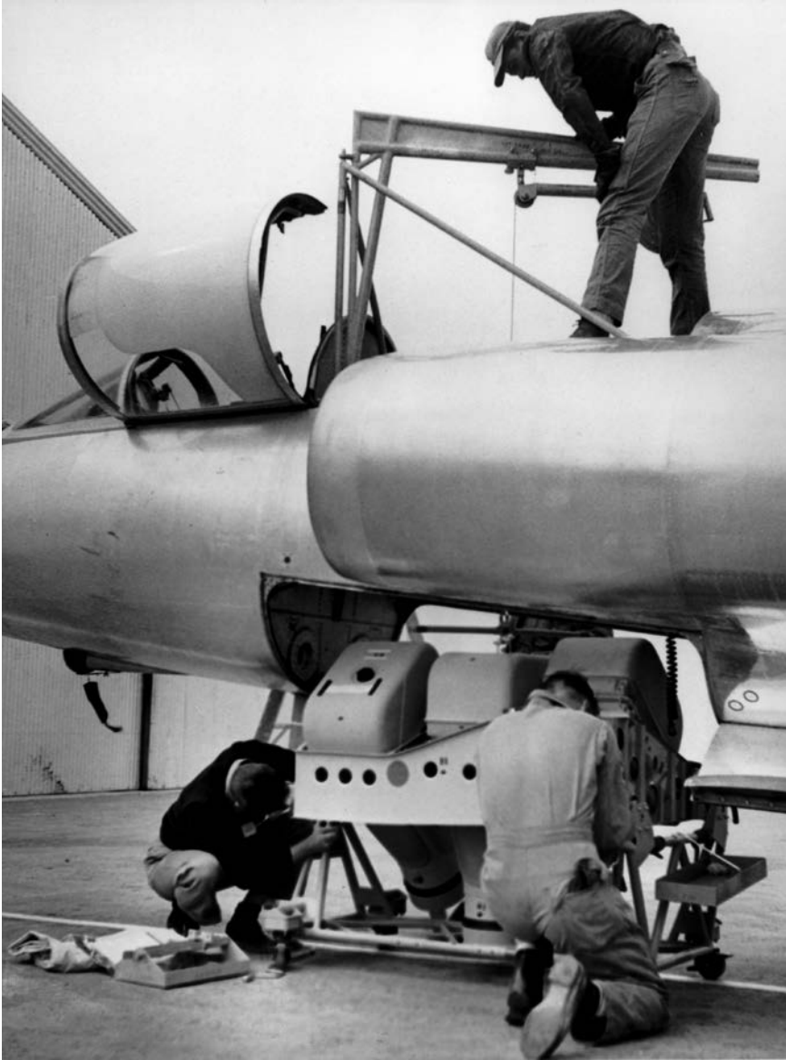
Technicians install a camera package in the Q-bay of a U-2A. (Lockheed Martin)
