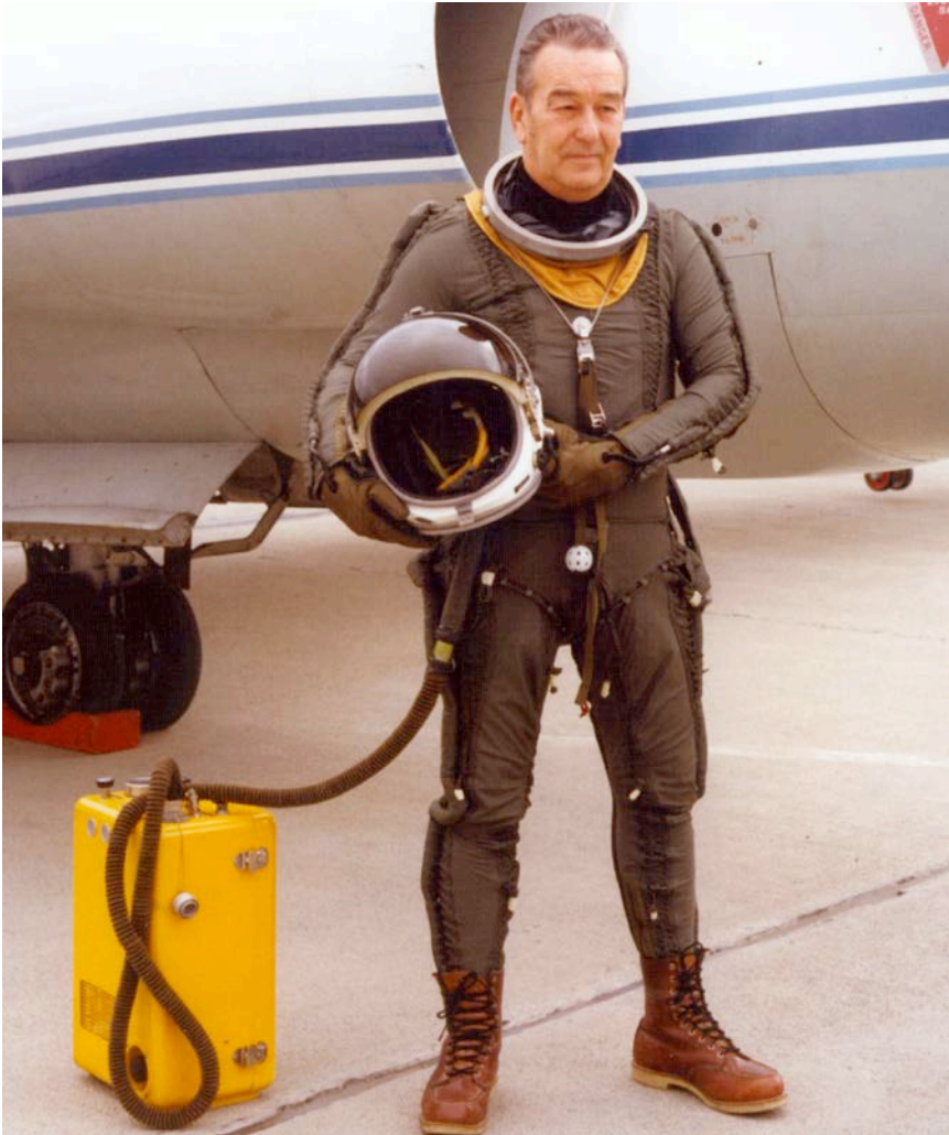
The S-100, worn here by NASA pilot Jim Barnes, was a hybrid of a partial-pressure suit and a full-pressure-type helmet. (NASA)
