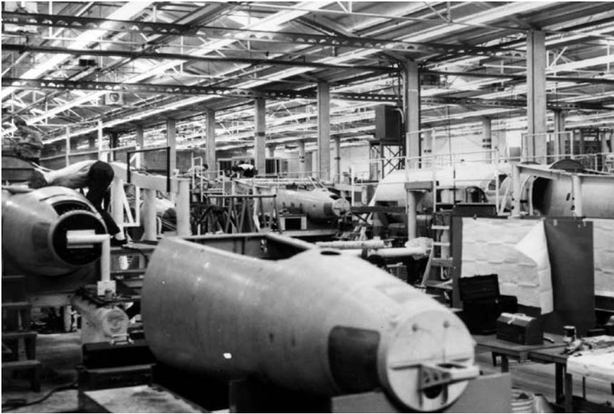
U-2 forward fuselage assemblies under construction. (Lockheed Martin)
