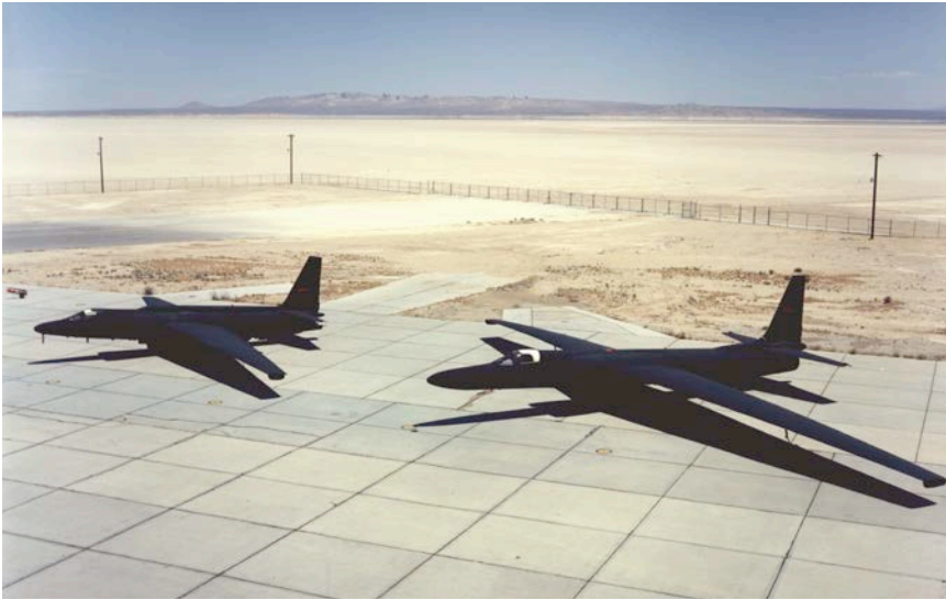
With its lengthened fuselage and wings, the U-2R, right, was significantly larger than the U-2C. (Lockheed Martin)
