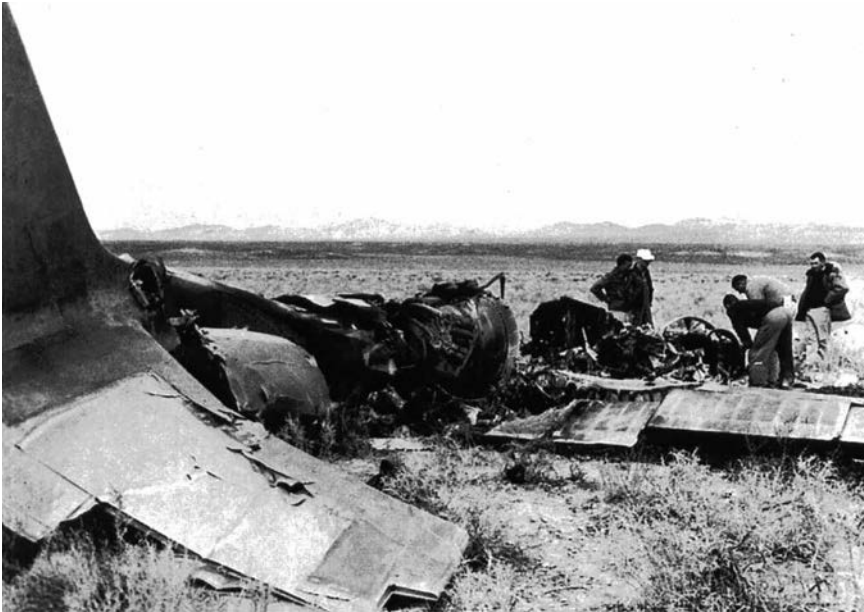
Article 341 crashed in a flat spin following a flameout at 72,000 feet. Lockheed test pilot Robert Sieker was killed. (CIA)
