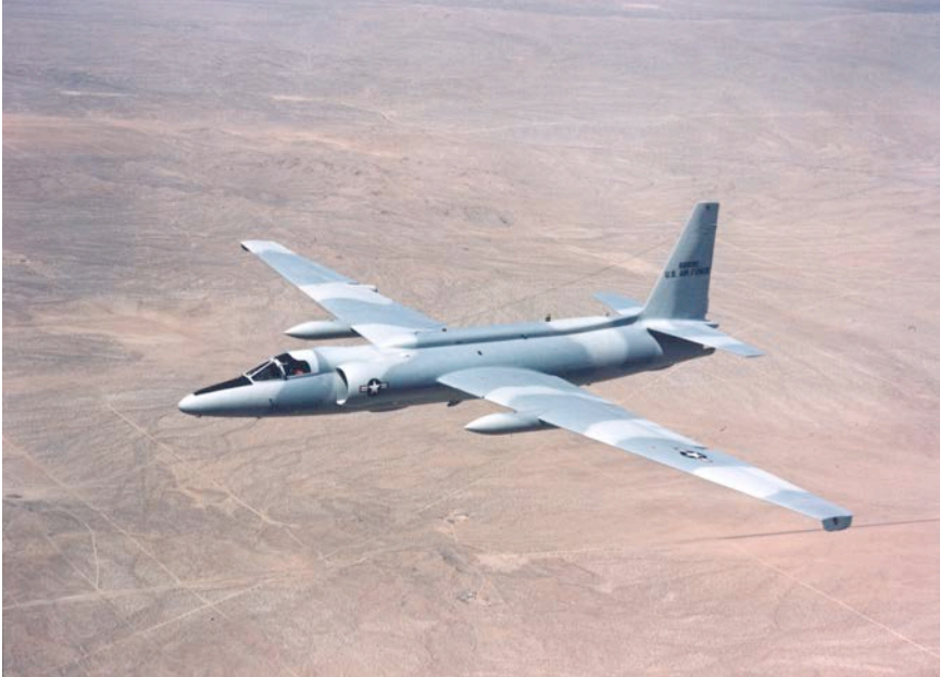
The U-2C had fluted inlets to accommodate increased airflow to the J75 engine and a dorsal spine housing additional equipment. Note the 100-gallon slipper tanks on each wing. (Lockheed Martin)
