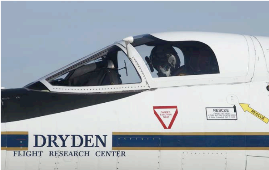
A painted sunshade limited visibility through the lightweight canopy. (NASA)
