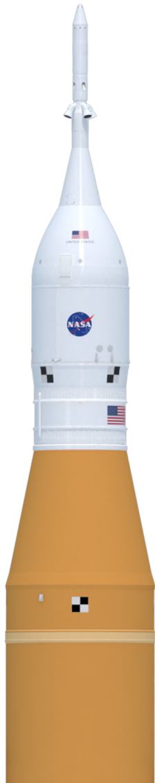
The Orion stage adapter, with volume for CubeSats, connects the SLS upper stage to the Orion Spacecraft.
