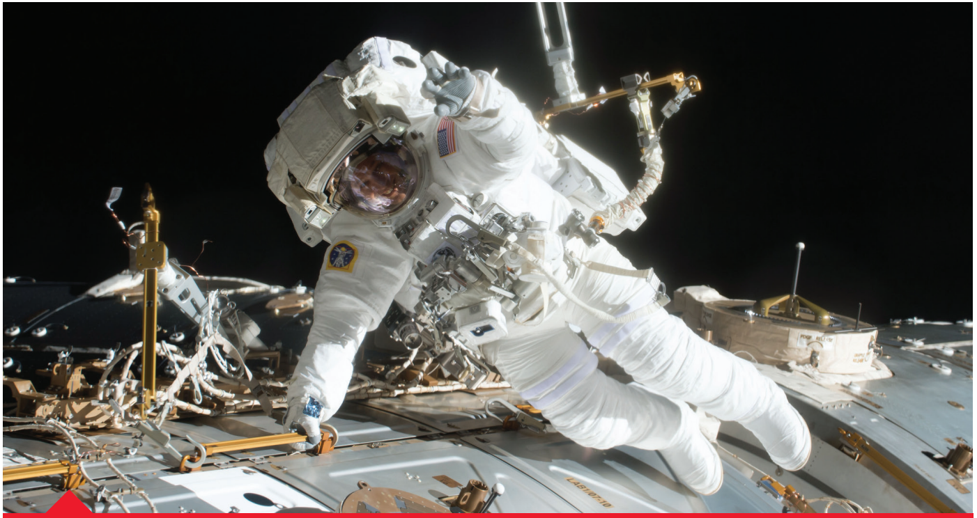
Air Force Colonel and NASA astronaut Jack Fischer works outside the U.S. Destiny laboratory module to attach wireless antennas during the 201st spacewalk in support of International Space Station maintenance and assembly. This was a short and unplanned contingency spacewalk whose primary task was the removal and replacement of a failed computer data relay box that controls the functionality of important station components such as solar arrays and radiators. Photo credit: NASA
