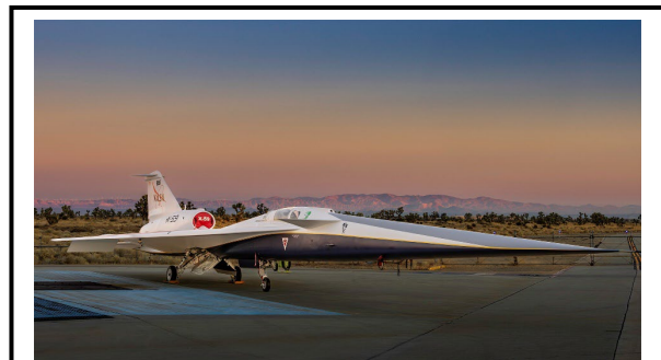
NASA's X-59 supersonic aircraft sits on the apron outside Lockheed Martin's Skunk Works. The X-59 seeks to make sonic booms quieter. Credit: Lockheed Martin Skunk Works
