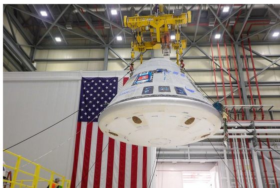
The Starliner crew module is shown here being hoisted in Boeing's Commercial Crew and Cargo Processing Facility at KSC in Florida on January 19, 2023, before being mated to a new service module for NASA's Boeing Crew Flight Test.
