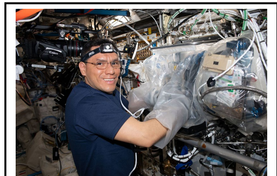
NASA Astronaut Frank Rubio, pictured here, uses a glovebag and services the BioFabrication Facility, replacing and installing components inside the research device, which is designed to print organ-like tissues in microgravity and learn how to manufacture whole, fully functioning human organs in space (September 25, 2023).
