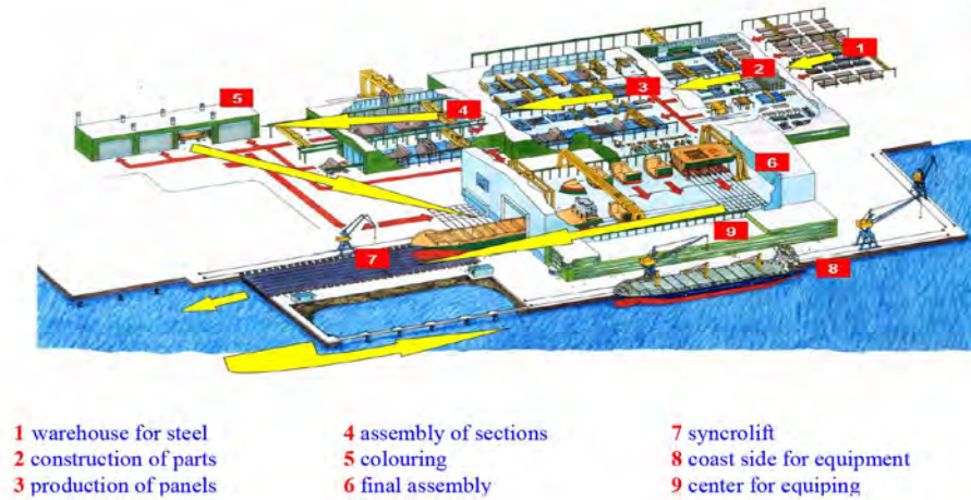
Figure 2 Modern prefabricated shipyard with following objects, transport roads and other infrastructure elements
