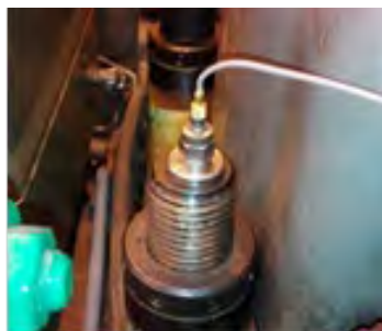
Figure 4 An example of accelerometer assembly on the Sulzer tightening bolt - direction V
