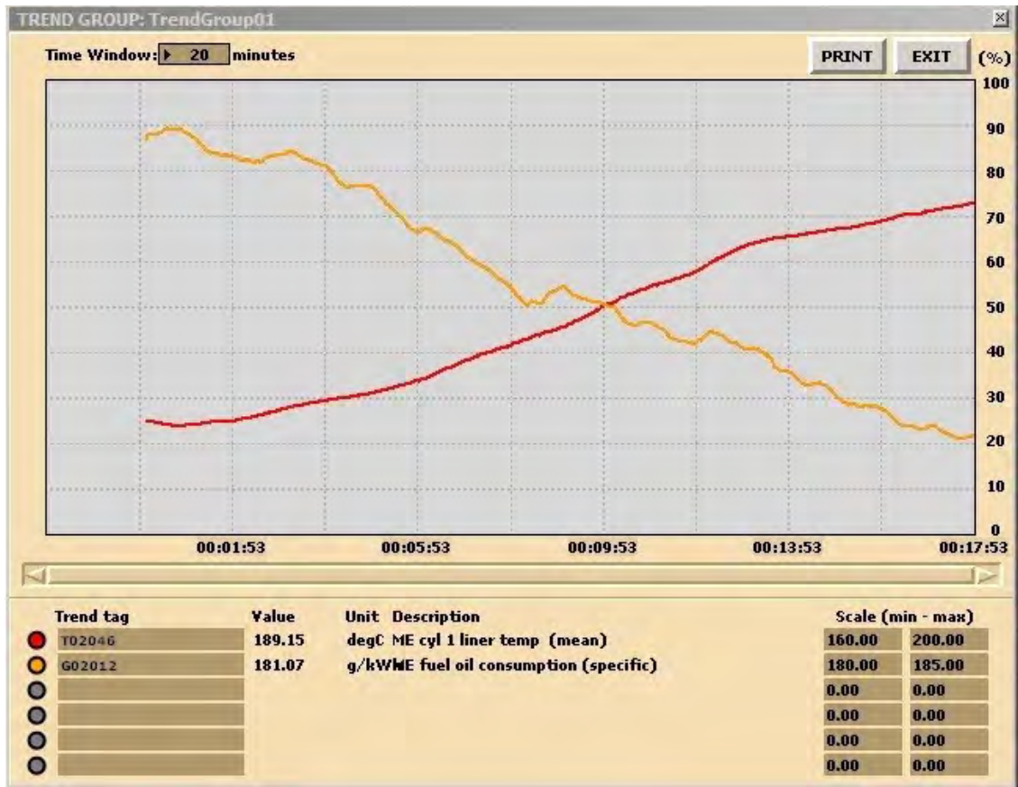
Figure 3 Trend of specific fuel consumption dependency on cylinder liner temperature on Kongsberg simulator [Kongsberg Norcontrol Engine Room Simulator]
