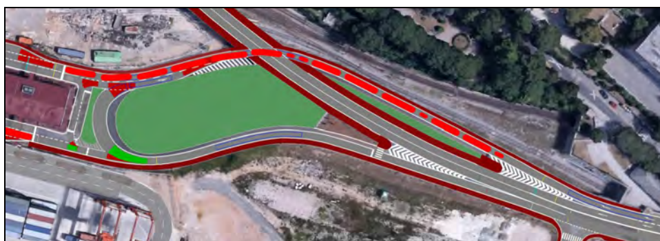
Figure 7 Presentation of congestion and boundary throughput of the access road (existing load) - Scenario 1
