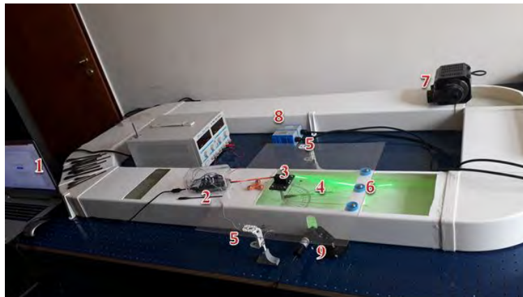
Figure 9 Measurement stand; 1 – computer, 2 – microcontroller, 3 – servomechanism, 4 – tested fin, 5 – strain gauges, 6 – ball bearings, 7 – water pump, 8 – flowmeter, 9 – laser
