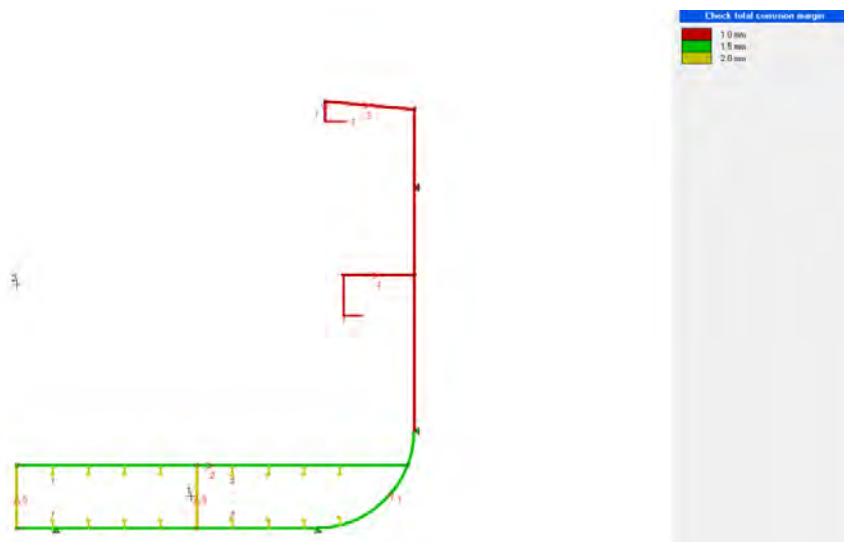
Figure 9 Corrosion margin of the ship in 25 years of activity
