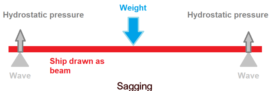
Figure 11 Representation of Sagging effect related to ship drawn as a girder
