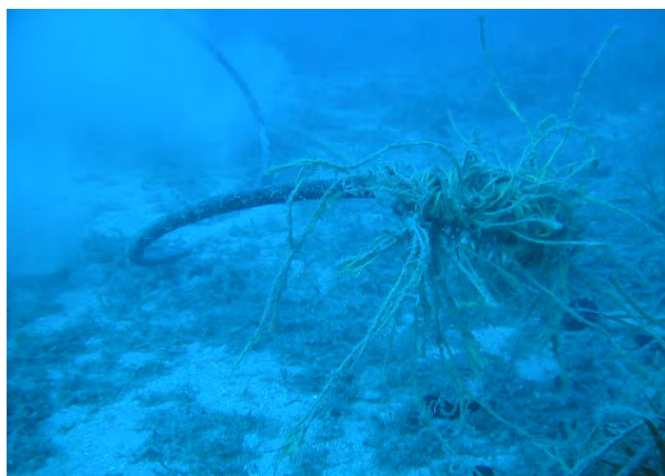
Figure 4 Optical cable breakage caused by anchoring
