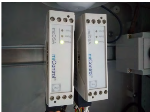
Figure 7 a) Drive controller mcDSA-45, b) miCAN-Stick2 converter
