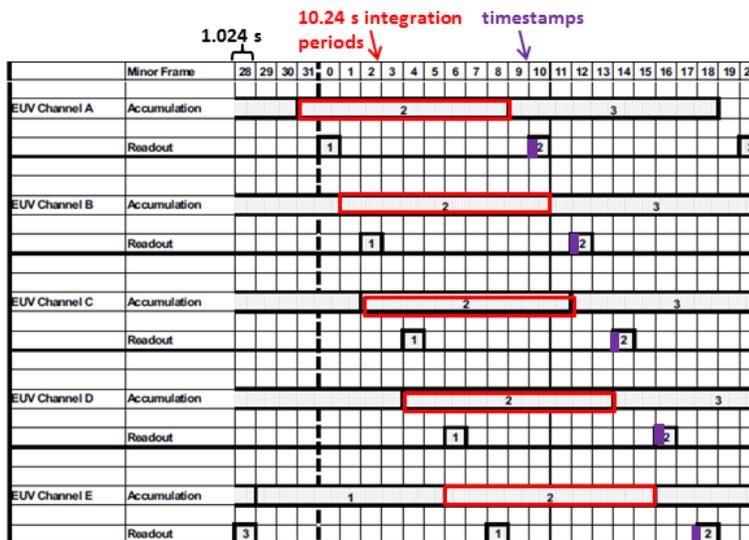
Figure 10: Sketch of EUVS instrument timing. Telemetry minor frames are 1.024 s. Integration is 10.24 s and timestamps occur 1.024 or 2.048 s after the end of the integration, depending on channel.
