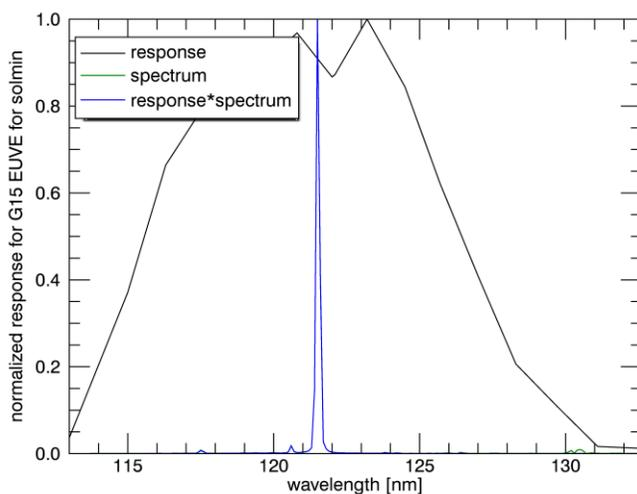
Figure 7: The EUVS-E responsivity, the LASP WHI quiet sun solar spectrum, and the convolved detector response for GOES-15.
