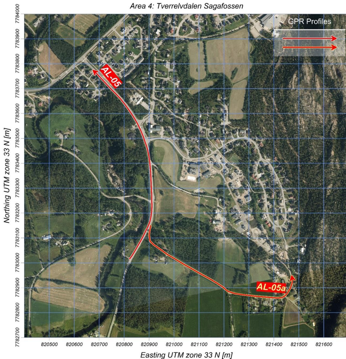
Figure 4.4.1: Positioning of Georadar profiles AL-05 and AL-05a collected at Tverrelvdalen Sagafossen area. Orthophoto: Vest Finnmark (Field-Group, 2023).
